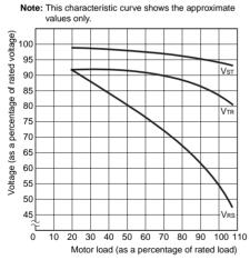
**Note:** For phase loss of phase R. V<sub>ST</sub>, V<sub>TR</sub>, and V<sub>RS</sub> indicate the motor terminal voltage at phase loss.
